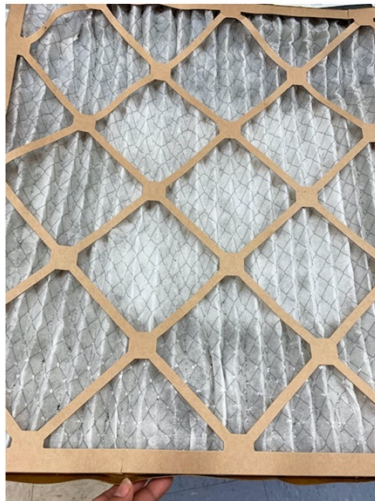
Figure 3. Air filters taken from Dr. Salazar's lab in rooms 442C and 442D. Pictures were taken on September 6, 2021 before the cleaning of the air ventilation system started in September 7, 2021. Pictures of the filters in rooms 442D and 442C show the blackened filter paper and black particles of diverse sizes.
