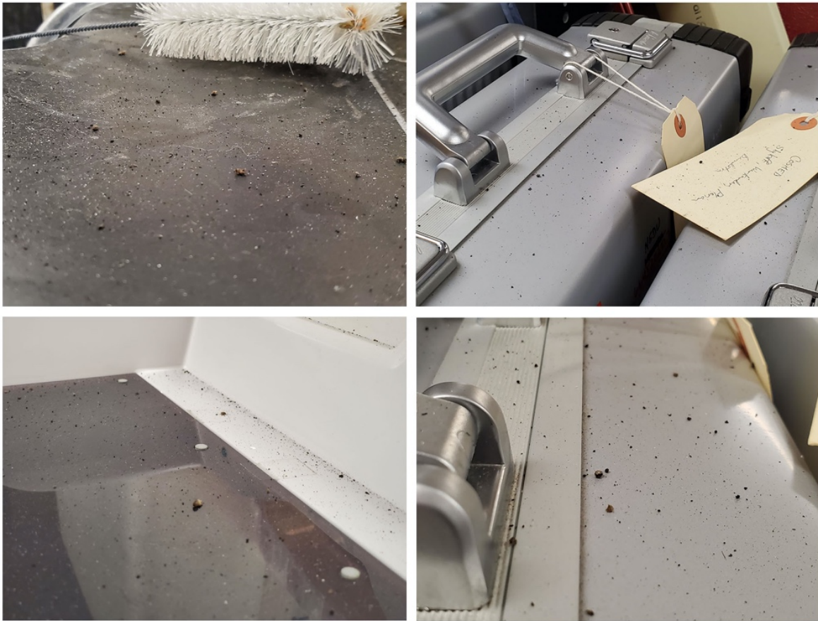
Figure 4. Example of black particles found on surfaces in the Sandels Building. Pictures were taken on September 7, 2021 the day when the cleaning of the air ventilation system started. Pictures show the black particles found on top of benches and equipment in Dr. Kim's lab in Room 440.
