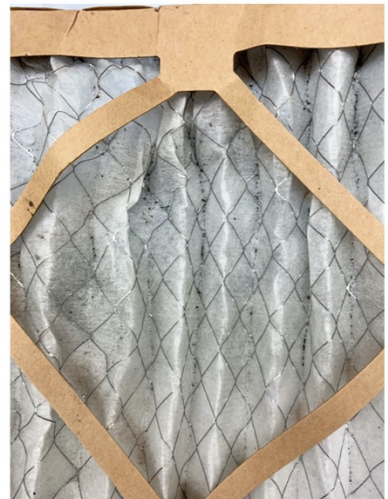
Figure 3. Air filters taken from Dr. Salazar's lab in rooms 442C and 442D. Pictures were taken on September 6, 2021 before the cleaning of the air ventilation system started in September 7, 2021. Pictures of the filters in rooms 442D and 442C show the blackened filter paper and black particles of diverse sizes.
